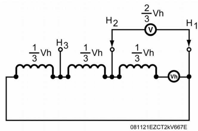
Figure 16. Buried CT in a Delta Transformer Illustration 2
