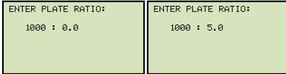
Type the second number using the keypad and then press the **[ENTER]** key. Continue to step g.
