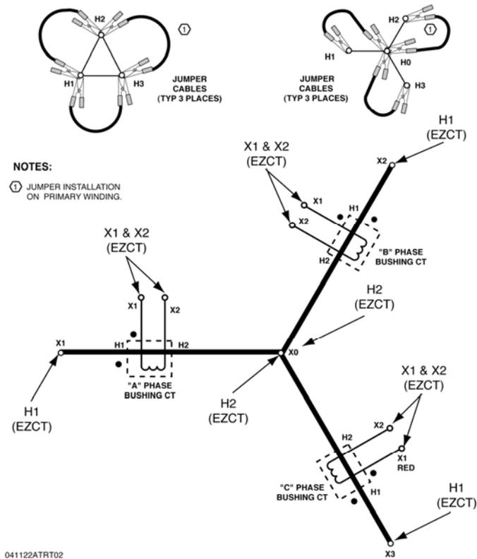
Figure 4. Bushing CT Connection on Y Transformer
