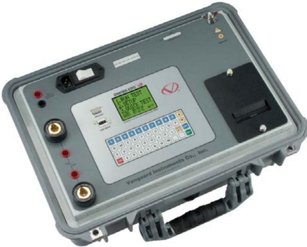
The DMOM-200 S3 is Vanguard's fourth generation, microprocessor-based, true DC micro-ohmmeter. It is designed for testing EHV circuit-breaker contact resistances, bushing contact joints, welding joints, or for any low-resistance measuring application. This high current and very lightweight (19.8 lbs/ 8.9 Kg) micro-ohmmeter is designed to meet the IEEE C57.09-1999 (5.15) requirement for testing circuit breaker contact resistance.
